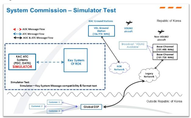
2.2.2 Second phase is designed to make best performance of interface among Key system, Simulator and aircraft via VDL ground station. This test will verify and confirm DATIS and PDC message format and message flow between Simulator and VDL active aircraft. The system configuration is as below.
