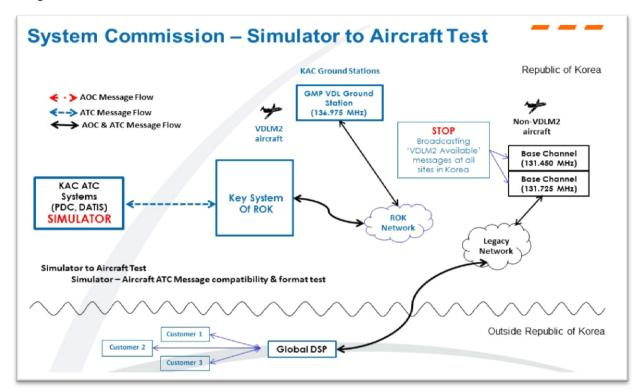
2.2.3 Final phase is designed to optimize Key system in operation regarding interface among Key system, Simulator and aircraft via all (8sites) VDL ground station activated while broadcasting "VDLM2 Available message" from ACARS transceiver. The system configuration is as below.
